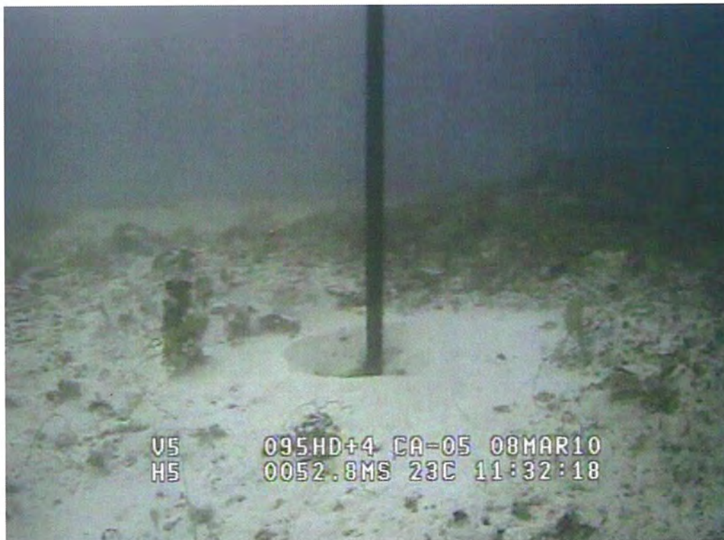
Figure 8. Image of bottom conditions during coring during the Great Barrier Reef Expedition, which shows the drill pipe coming down from the vessel-mounted rig. Rock cuttings are visible around the borehole. The coring debris is thickest in the immediate vicinity of the borehole (within a metre or two), and then tail off with distance from the borehole. Fine cuttings are generally dispersed by currents. Note that this image demonstrates coring using traditional drilling methods. Coring using a seafloor drill will produce less volume of cuttings in comparison.
