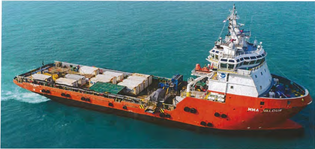
Figure 2. Multipurpose Vessel MMA Valour, the proposed project vessel. A seafloor corer will be launched over the starboard side the vessel, slightly forward of midship. https://www.mmaoffshore.com/vessel-fleet/mma-valour .
