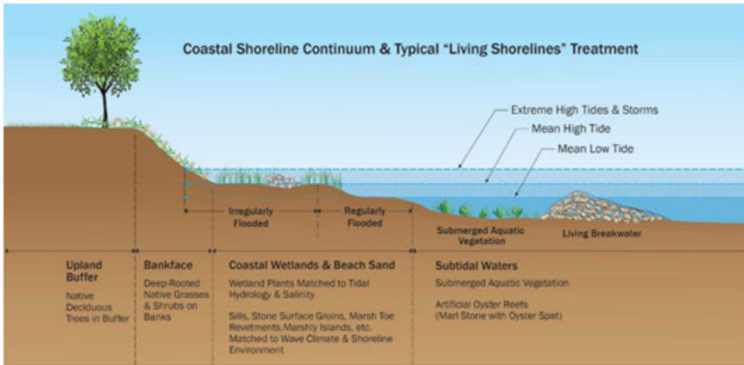
Figure 5.4.8. Nature-based solutions for shoreline stabilization via a “Living Shorelines” approach. (Source: Adapted from NOAA, 2016)
