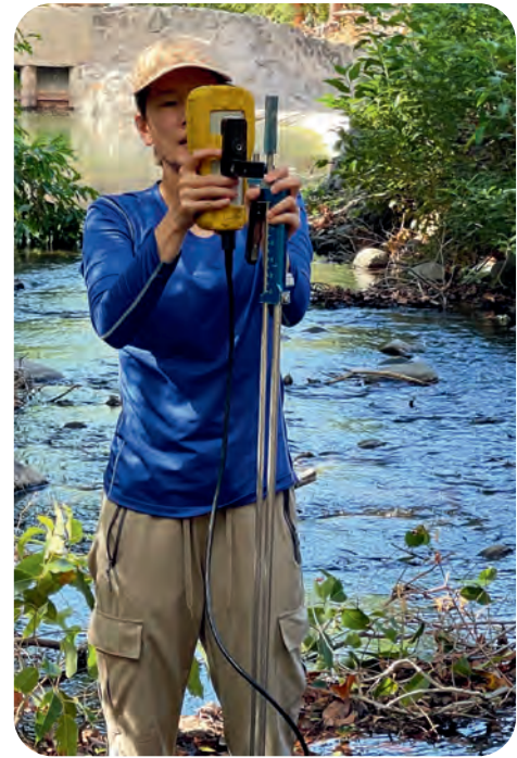
Cody Chacon, Hydrologist, takes a stream flow measurement at Olowalu Stream, Maui
