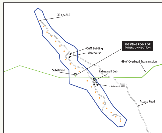
INTERCONNECTION ROUTE: Point of interconnection is located at the existing KWP I substation and the interconnection route will remain the same
