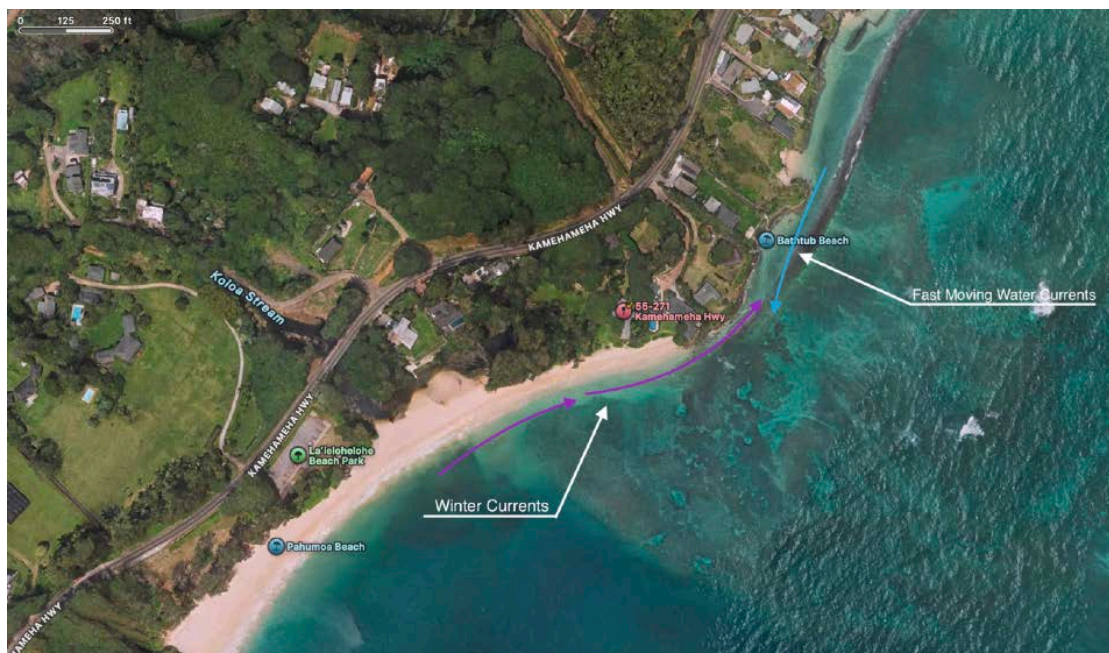
Figure 3-7: Currents Allowing Sand Accumulation at "Bathtub Beach"
