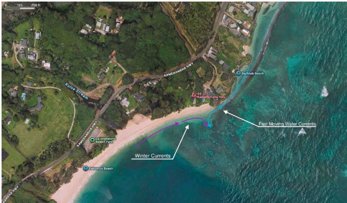
Figure 3-8: Competing Currents not Allow Sand Pass Point
