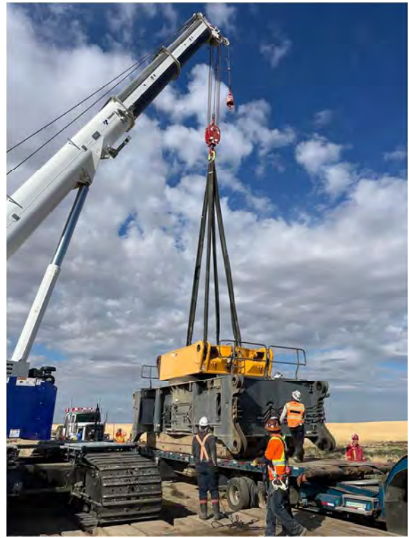
Figure C-7. Assembly of Liebherr LR 11000 Crawler Crane (Source: Buckner Heavylift)
