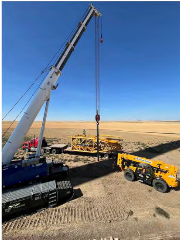
Figure C-14. Assembly of Liebherr LR 11000 Crawler Crane (Source: Buckner Heavylift)
