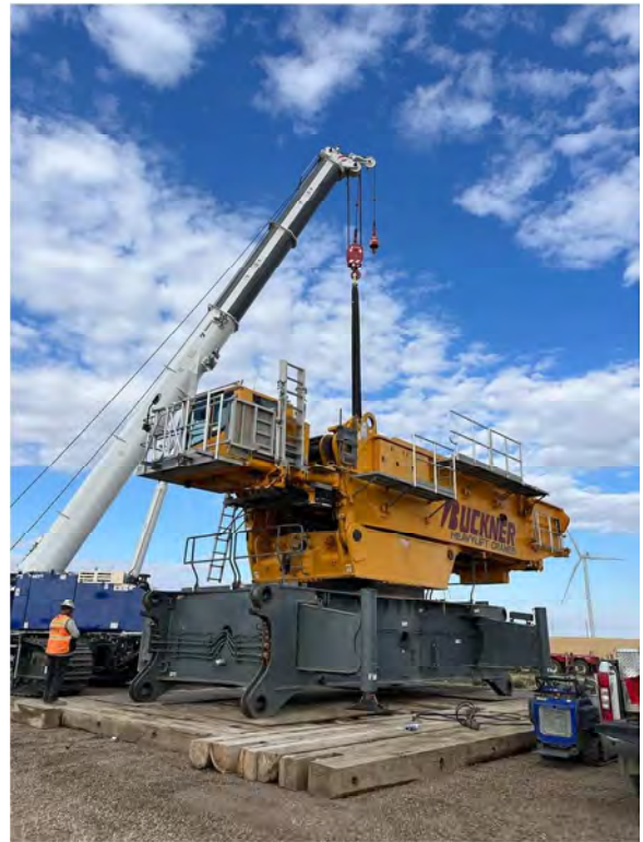
Figure C-9. Assembly of Liebherr LR 11000 Crawler Crane (Source: Buckner Heavylift)
