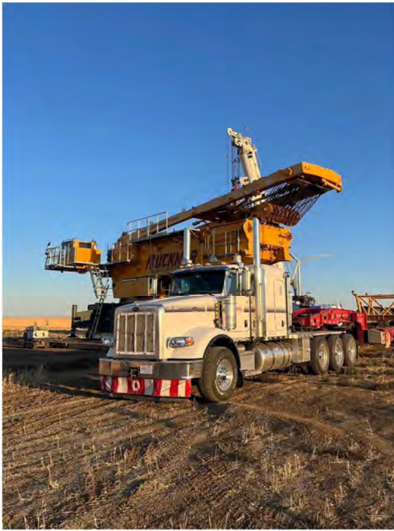
Figure C-6. Assembly of Liebherr LR 11000 Crawler Crane (Source: Buckner Heavylift)
