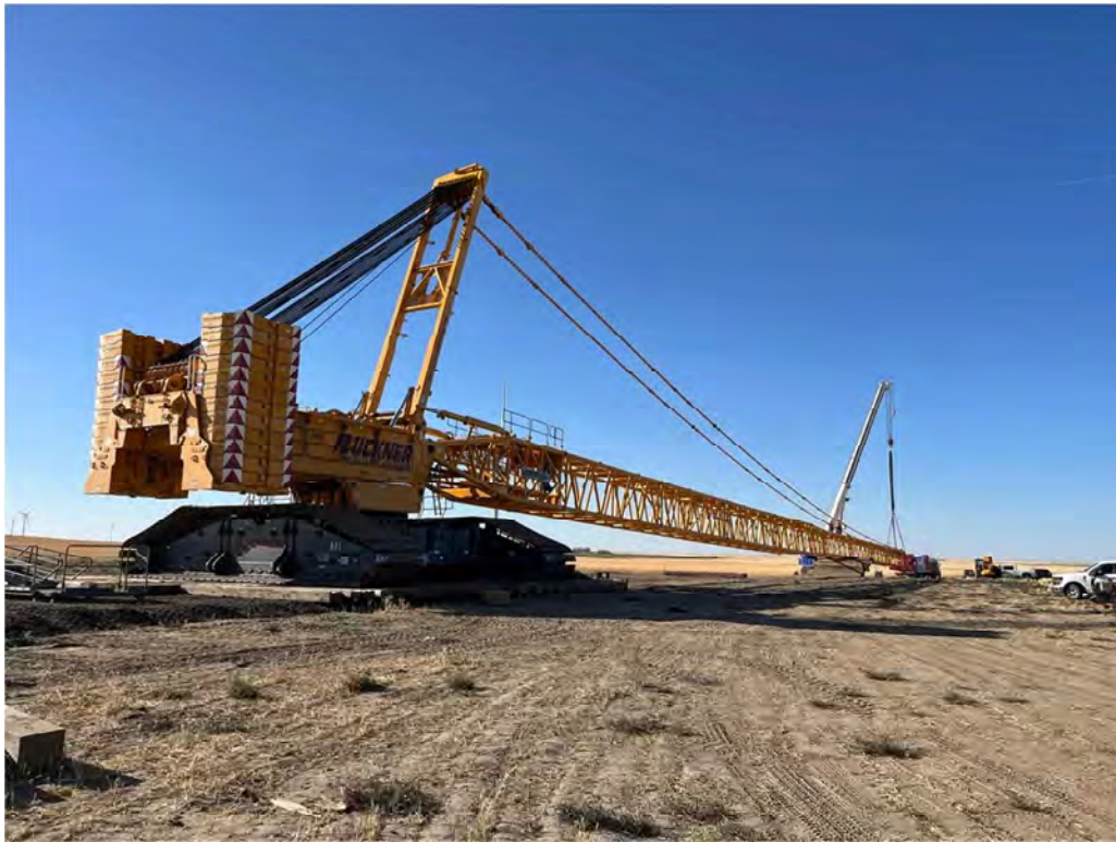
Figure C-18. Assembly of Liebherr LR 11000 Crawler Crane (Source: Buckner Heavylift)
