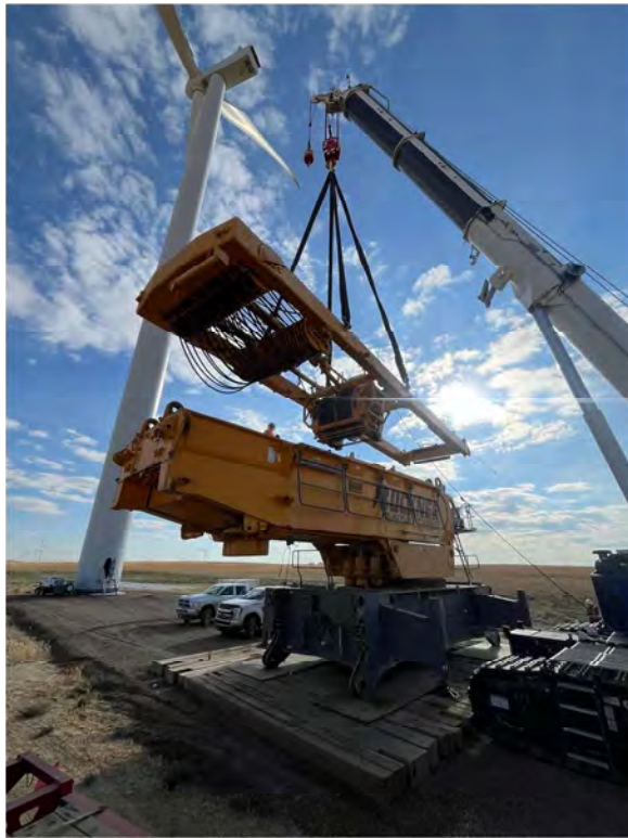
Figure C-10. Assembly of Liebherr LR 11000 Crawler Crane (Source: Buckner Heavylift)
