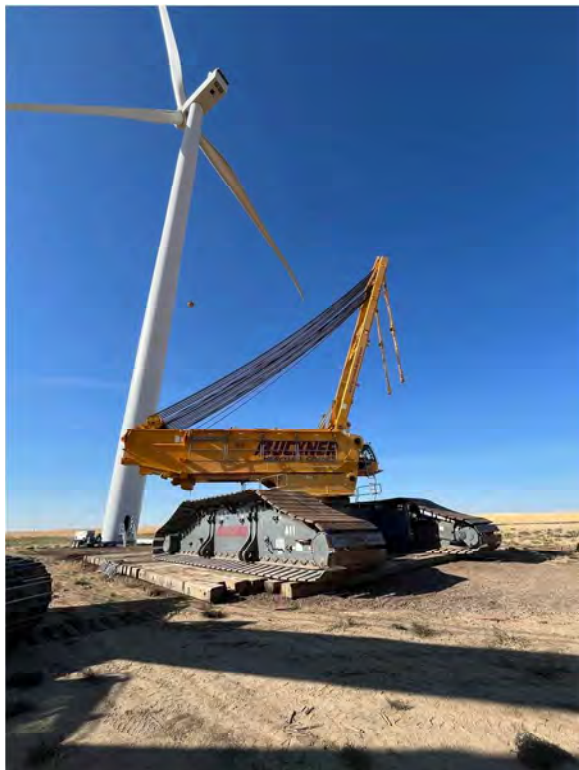
Figure C-12. Assembly of Liebherr LR 11000 Crawler Crane (Source: Buckner Heavylift)
