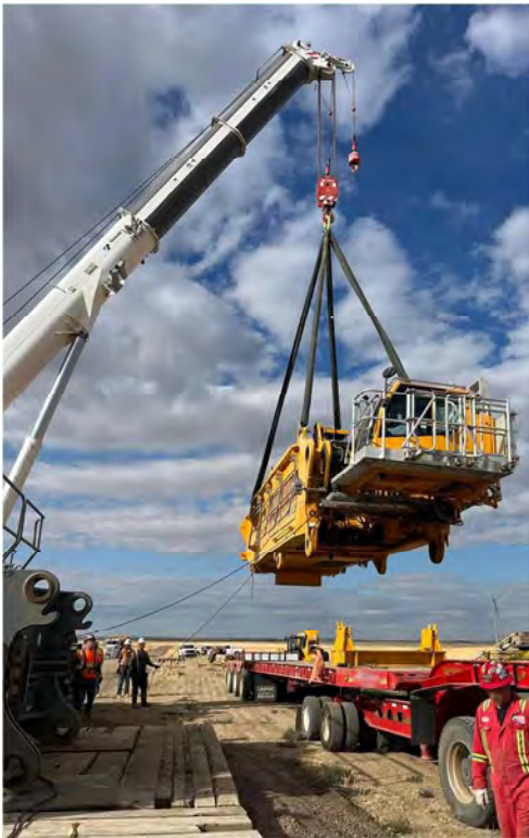
Figure C-8. Assembly of Liebherr LR 11000 Crawler Crane (Source: Buckner Heavylift)
