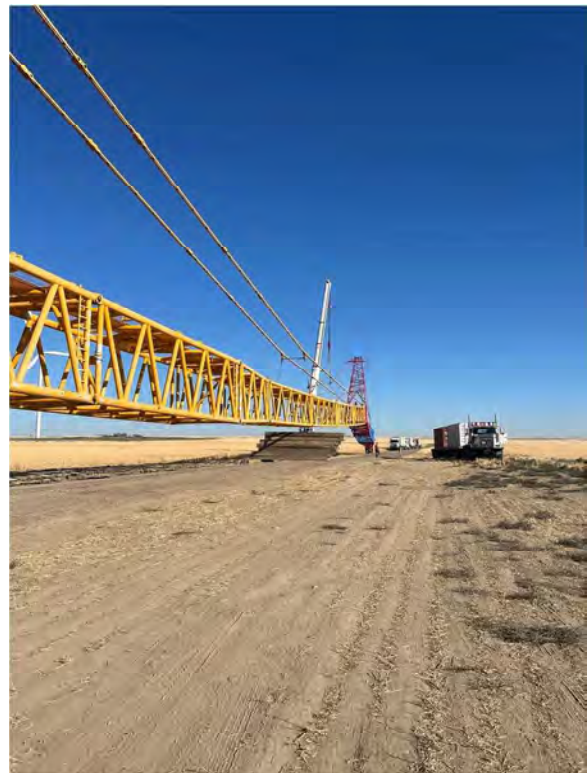
Figure C-17. Assembly of Liebherr LR 11000 Crawler Crane (Source: Buckner Heavylift)
