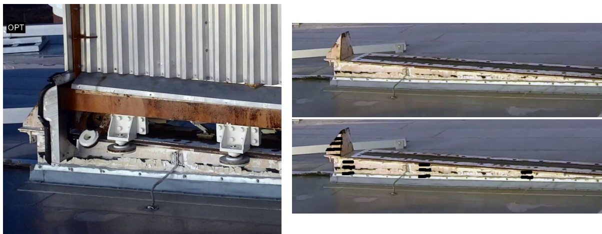
Figure 8: [Left] zoom-in view of the guide rail under the Open state. Our webcam can zoom-in five times closer than this. [Right] The proposed markers on the rail. We put black lines every 0.25 inches.
