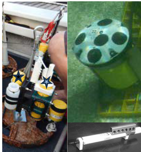
Instrument Deployment #2/#3: One Nortek Signature 1000 (right); One RBR Virtuoso Dwave Logger (left; black star); One Seabird MicroCAT (bottom right); One RBR Tu (middle-bottom; blue star) Deployed Together on a Ballasted Frame with a Vertical Bar for Securing the Sensors
