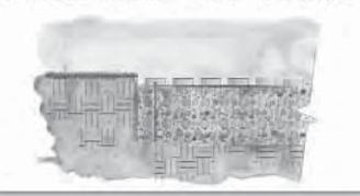
For Grasspave<sup>2</sup>: Compacted sandy gravel road base placed above compacted subgrade, 95% modified.
