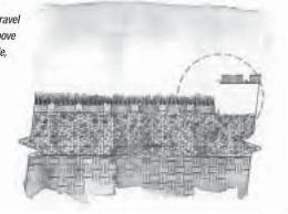
92 percent void space for the best root development and grass coverage (Grasspave<sup>2</sup>) and the most volume available for desired fill (Gravelpave<sup>2</sup>). Most other plastic pavers come in rigid unit blocks, which are cumbersome to install and difficult to cut and shape. Grasspave<sup>2</sup> and Gravelpave<sup>2</sup> rolls are considered
